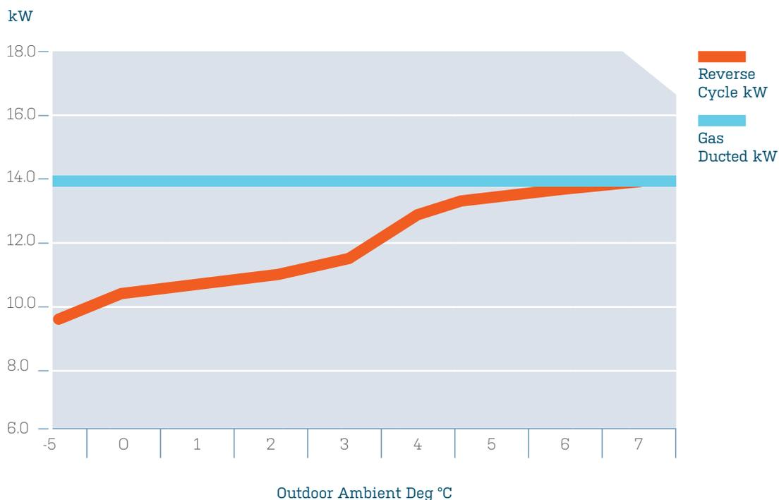
As the outdoor temperature drops, ducted reverse cycle heaters become less effective. Kaden's gas ducted heater maintains its' power output (shown in graph above) to keep you and your house toasty all through winter.
