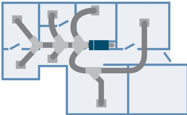
A gas ducted heater works by taking air from within the house, heating, then distributing through a series of duct work and outlets in the roof or floor.
